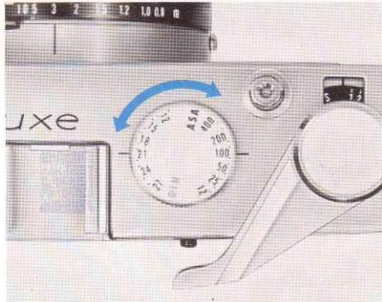
2 Next, note the filmspeed (ASA or DIN) rating of the film you are using, and turn the filmspeed dial 17 so that the proper number comes into alignment with the film-speed index mark 14. If you fail to make this important adjustment, your entire film may be wasted through incorrect exposure.
